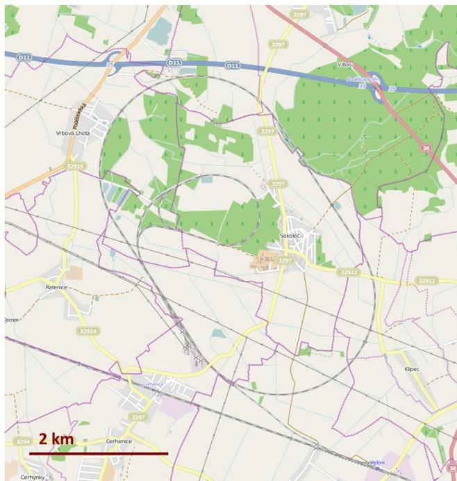
Yes, this is real... About 50km east of Prague there is a 13.25km oval of track which is used for testing, amongst other things, 230km/h tilting trains. Rail operators from all over Europe use it. More at [https://en.wikipedia.org/wiki/Velim\\_railway\\_test\\_circuit](https://en.wikipedia.org/wiki/Velim_railway_test_circuit) where you'll find pictures of a Class 92 under test.
